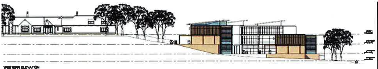
Fig. 71 The proposed development, seen from the west, with manor house at left. New buildings will be on the lower southern slope, and roof heights will not exceed those of the manor house.
